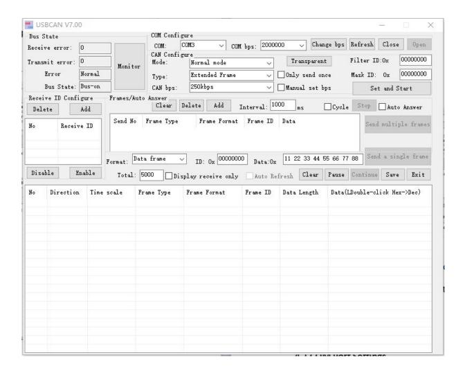
According to the CAN bus selecting frame type and set CAN baud rate, point solution set and start button, the CAN bus and the equipment the communication.
