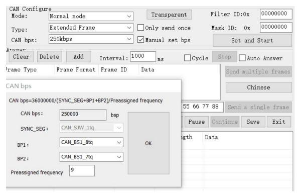
The top position CAN baud rate calculation formula, and at the same time set phase buffer 1, phase buffer 2, and preassigned frequency is ok
